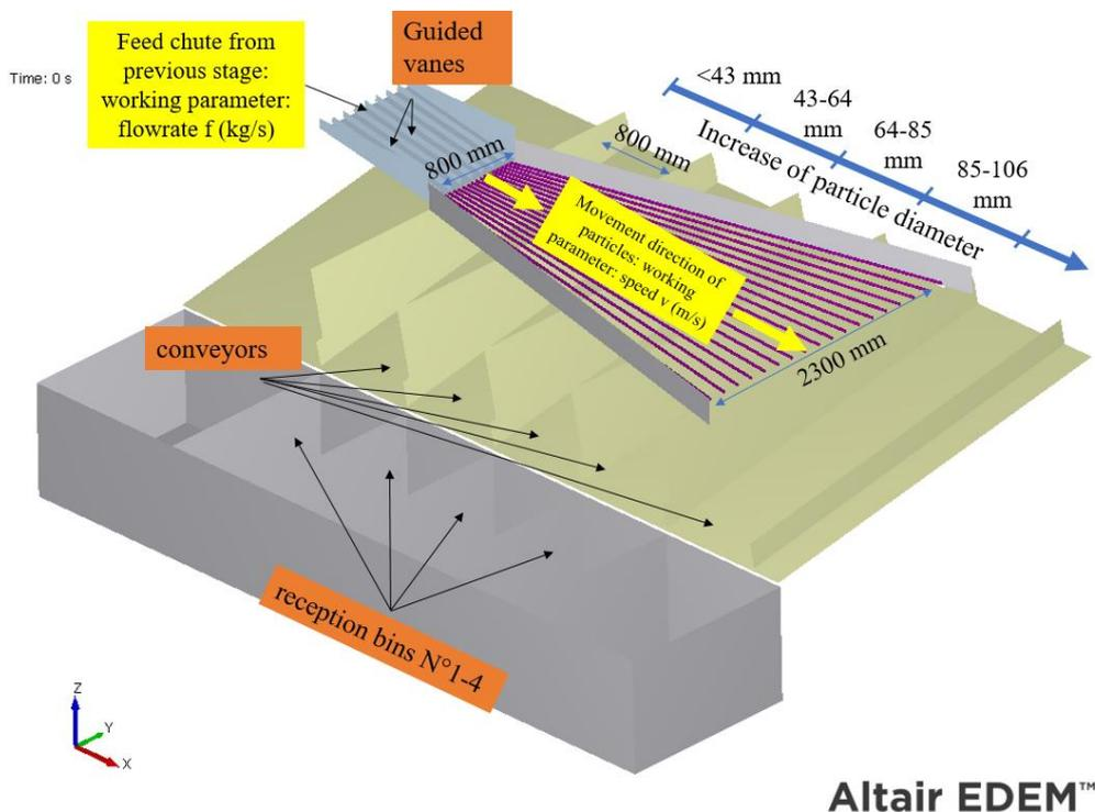
**Figure 1.** Schematic diagram of the working principle and related parts
