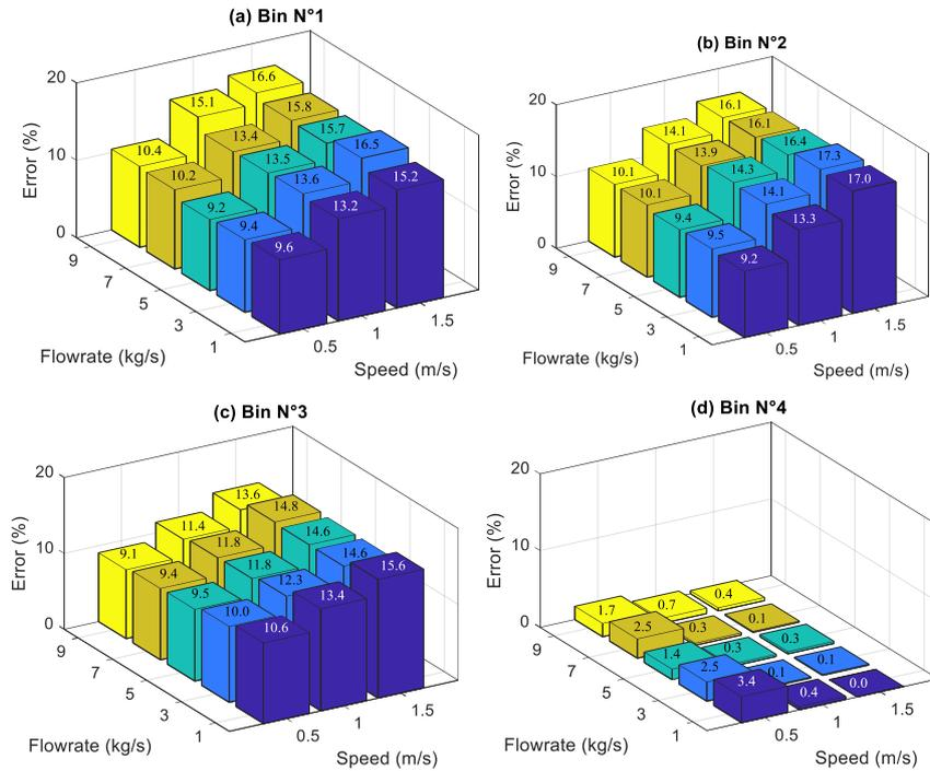
Figure 3. Errors of each sizing bin in varying moving speeds and flowrates (a) Bin N°1, (b) Bin N°2, (c) Bin N°3, and (d) Bin N°4
