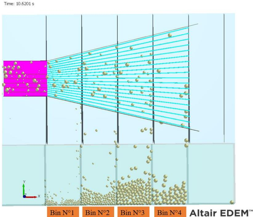
**Figure 2.** A capture screen for visualization of particles and equipment during simulation: the smallest particles were collected in Bin N°1, largest particles were collected in Bin N°4
