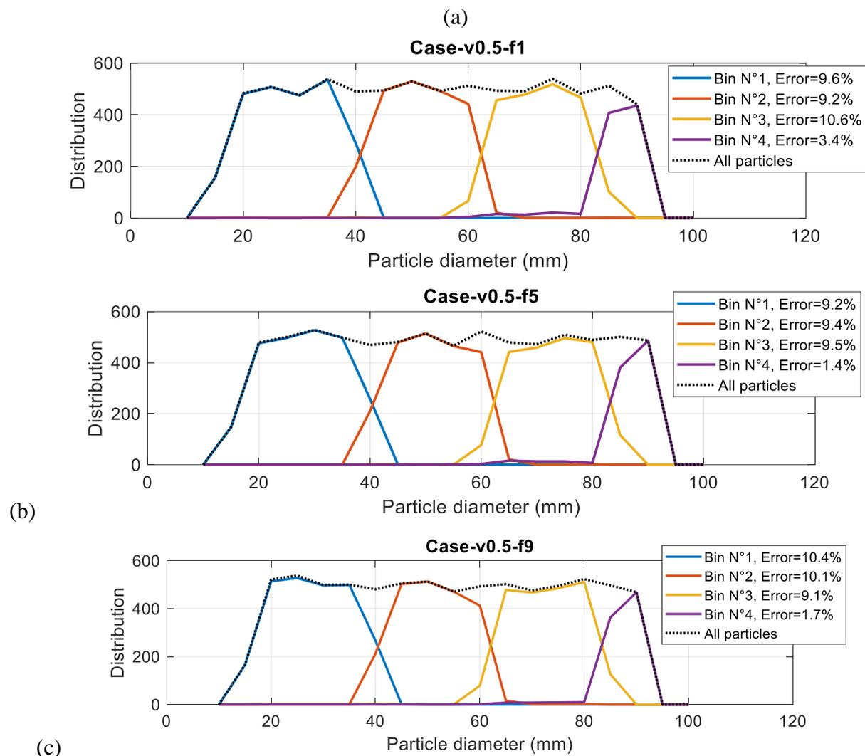
**Figure 5.** Effect of flowrate on sizing performance: histogram distributions of particles after finishing the process (1000kg of fruits): (a) Case-v0.5-f1, (b) Case-v0.5-f5 and (c) Case-v0.5-f9. In each figure, the histograms of all particles and of each sizing bin are shown, including corresponding errors
