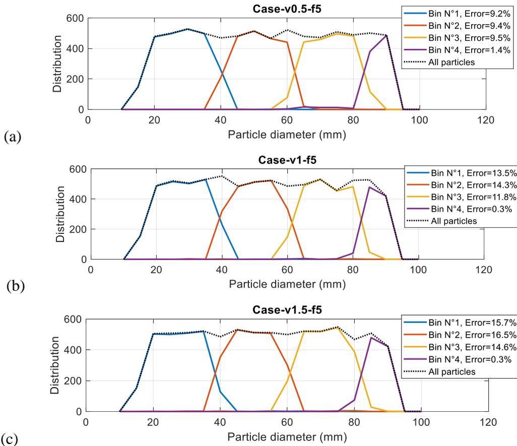
Figure 4. Effect of moving speed on sizing performance: histogram distributions of particles after finishing the process (1000 kg of fruits): (a) Case-v0.5-f5, (b) Case-v1-f5, and (c) Case-v1.5-f5. In each figure, the histograms of all particles and of each sizing bin are shown, including corresponding errors
