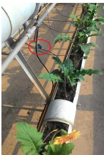
Figure 3. Setting up a light sensor
