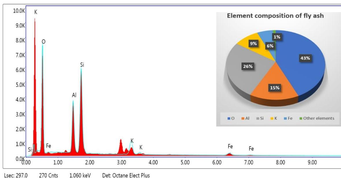
Figure 4. Chemical composition of fly ash by EDX technique
