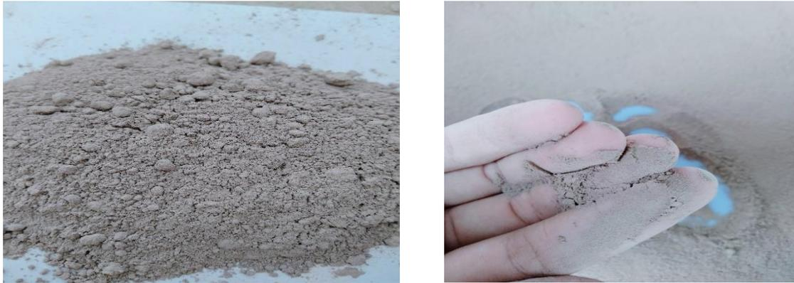
**Figure 1.** Fly ash collected from an ESP system at the Mong Duong 2 thermal power plant
