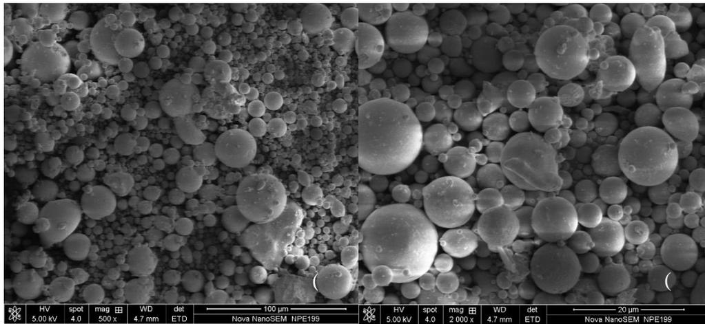
**Figure 3.** Scanning electron micrographs of the fly ash at (a) 500x and (b) 2000x magnification
