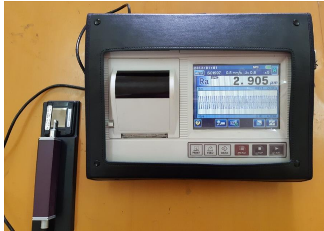
Figure 5. Mitutoyo Surftest RJ-210 test
